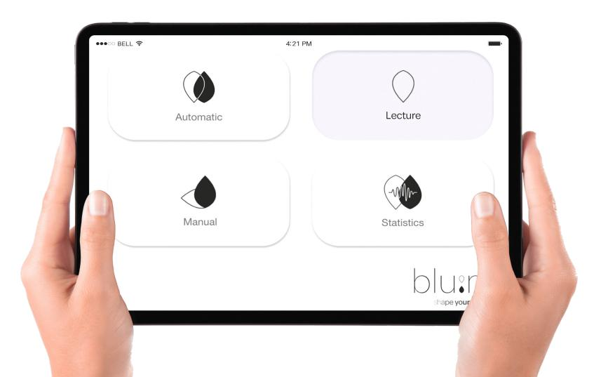
An interactive device mounted on the wall of the classroom allows the users to interact with the system. It can be used to turn the system on or off, change the system's setting, adjust any of the panels, and view the current sound levels in the room that are displayed on a graph.
